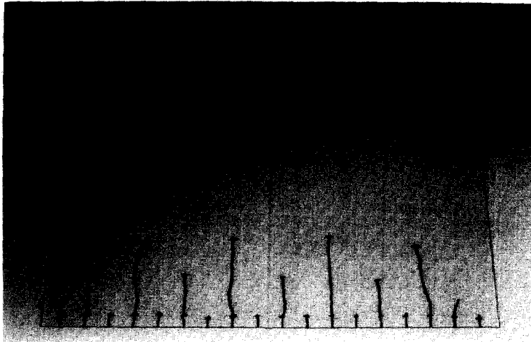
Fig. 7. Crack regime for plate with initial cracks; crack ends are marked at the end of the experiment.
